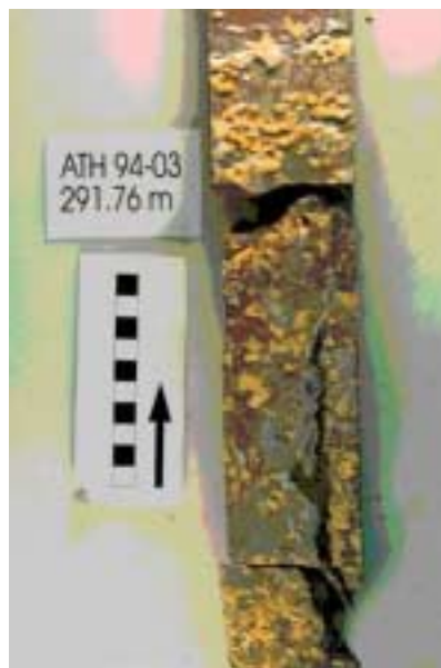
Figure 2. (bottom) Native sulfur crystals line a vertical fracture in bituminous laminites of the Methy (Winnipegosis) Formation, NE Alberta (sample from 291.8 m depth, drill hole ATH 94-03, Lac Minerals). Native sulfur records fracture controlled inflow of saline brines and reduction of sulfate.
